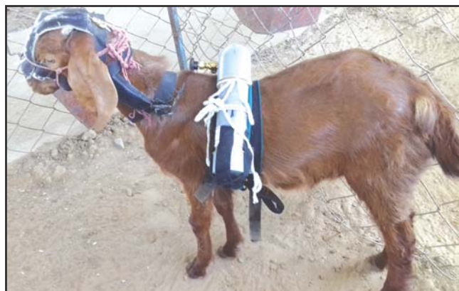
Lamb and kid with SF 6 assembly for methane estimation
